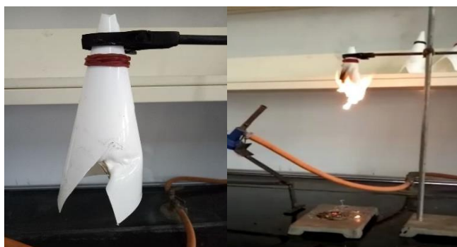
Fig 6 Shrinkage with burn mark after first flame and fire spread after 50 secs (BS1)
