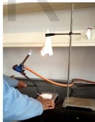
Fig 5 Reaction to fire on backsheet material
